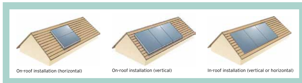
Different mounting methods for auroTHERM and auroTHERM plus flat plate solar collectors.
